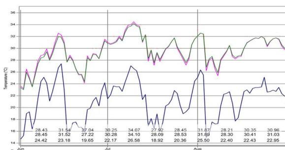
Fig. 7. Simulation result – Comparison of the effect of extruded polystyrene insulation and insulating plaster on the interior temperature in the polyclinic from Oravita – summer (Keller *et al.*, 2016)
