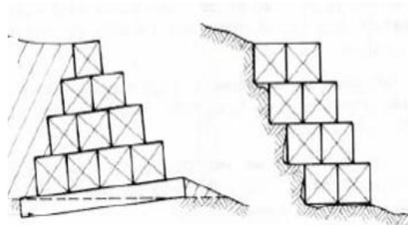
**Fig. 9.** Cage-walls - arrangement of cages (Facciorosso *et al.*, 2011)
