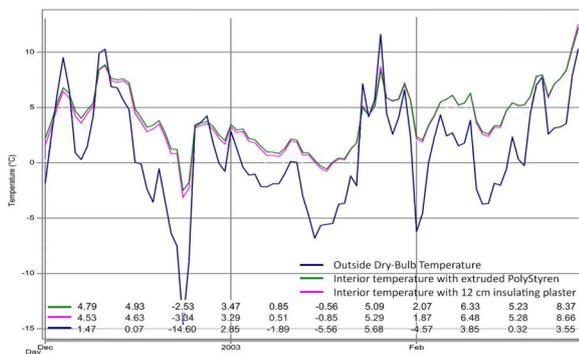
Fig. 6. Simulation result – Comparison of the effect of extruded polystyrene insulation and insulating plaster on the interior temperature in the polyclinic from Oravita – winter (Keller *et al.*, 2016)
