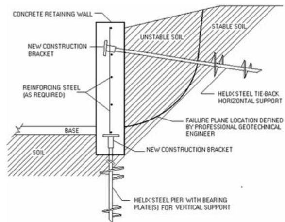
**Fig. 8.** Consolidation of an existing retaining wall by means of a steel tie (<http://southcoasthelix.com/about.html> - 02/05/16).
