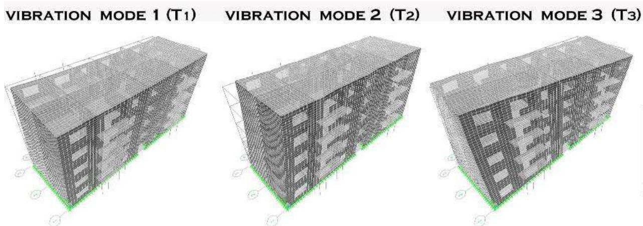
Fig. 5. Vibration modes and periods of original structure
