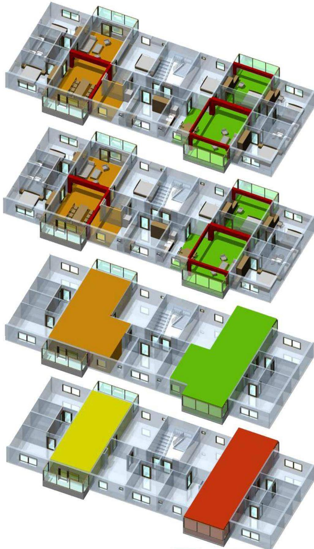
Fig. 3. Horizontal reconfiguration by coupling two apartments
