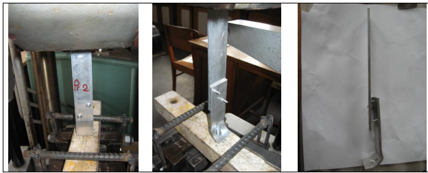
Fig. 8 – Failure mode by hole enlarging and nut passing through it and also by self-tapping screws rupture (for type 4 element)
