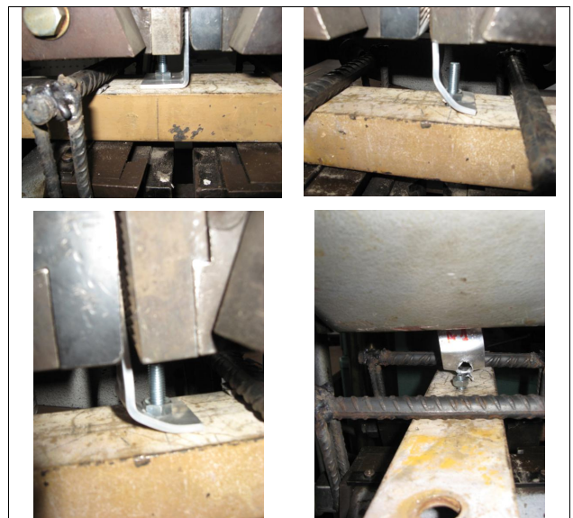
Fig. 6 - Failure mode by hole enlarging and screw nut passing through it (for type 1 element)
