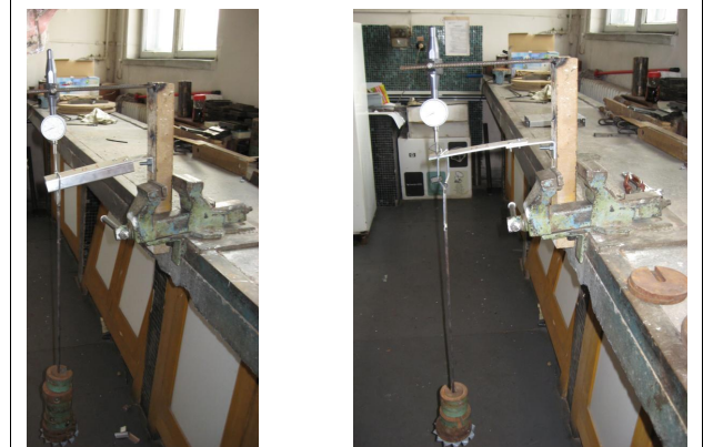
Fig. 11 – bending of the elements (for types 4 and 5 elements)
