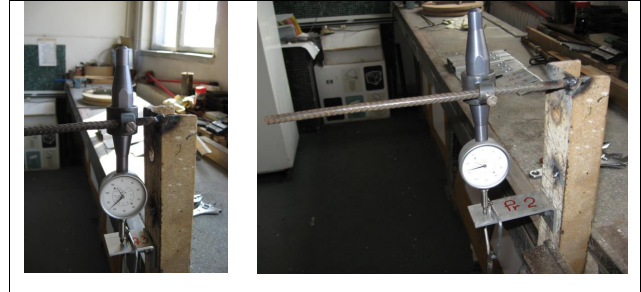
Fig. 10 – bending of the elements (for types 1 and 2 elements)
