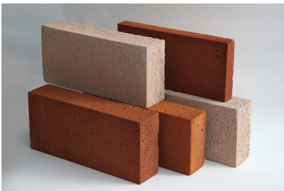
Fig. 2. Photo of ACP average density of 0.6 g/cm³ in the form of bricks and tiles.
