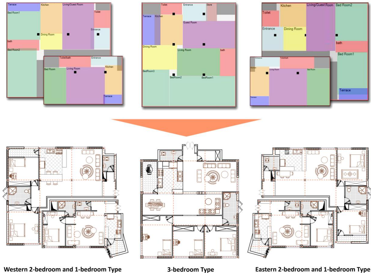
Fig. 10. Redesigned plans for the 5 plan types available in the case study using PSO algorithm.
