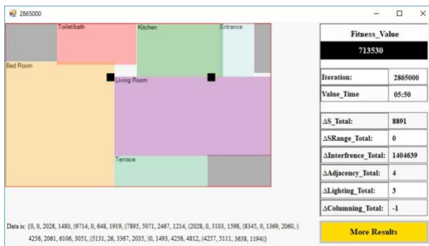
Fig. 8. A sample of the second step solution of the algorithm implementation for a western 1-bedroom plan.
