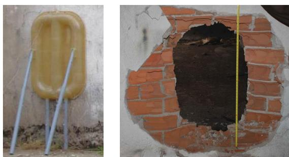
**Fig. 1.** Explosive Wall Breaching systems and their effects on masonry wall (Moldovan *et al.*, 2015)
