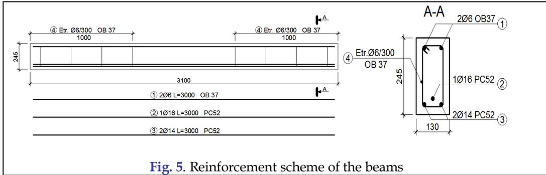
Fig. 5. Reinforcement scheme of the beams
