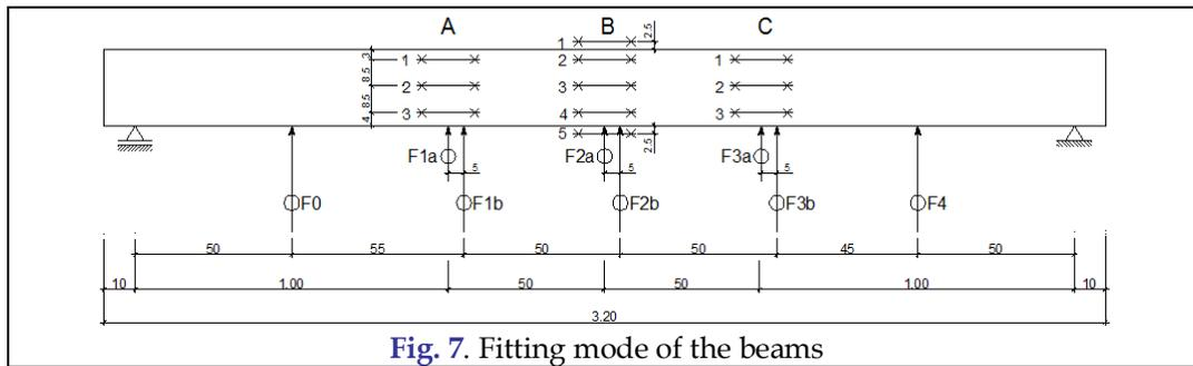
Fig. 7. Fitting mode of the beams
