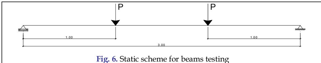
Fig. 6. Static scheme for beams testing
