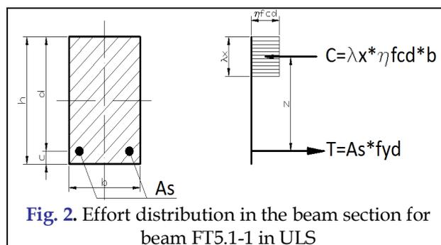
Fig. 2. Effort distribution in the beam section for beam FT5.1-1 in ULS
