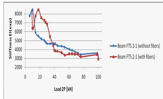
Fig. 9. Stiffness evolution (EI) of the beams
