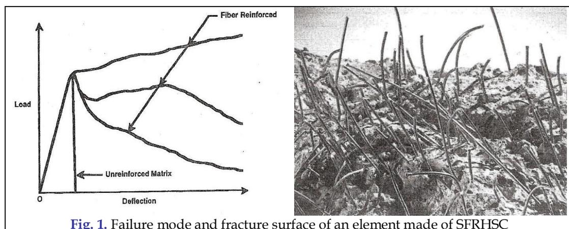
**Fig. 1.** Failure mode and fracture surface of an element made of SFRHSC
