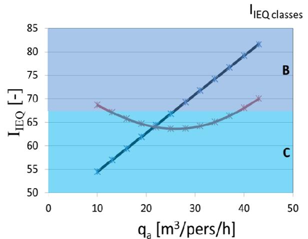
Fig. 6. Variation of the indoor environment quality depending on the fresh airflow: a) the fan placed outside of the apartment b) the fan is placed within apartment
